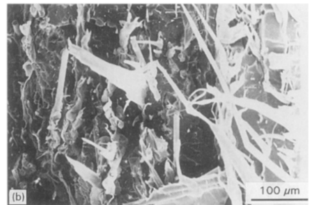
Figure 6 (a) SEM micrograph of the fracture surface of PP/33% LCP blend. A higher magnification of (b) skin layer and (c) core section of micrograph shown in (a).
