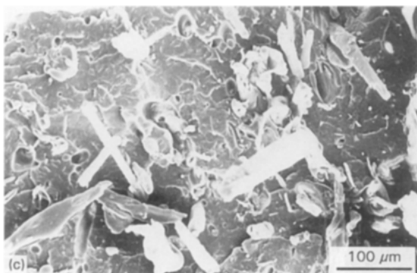
Figure 6 (a) SEM micrograph of the fracture surface of PP/33% LCP blend. A higher magnification of (b) skin layer and (c) core section of micrograph shown in (a).
